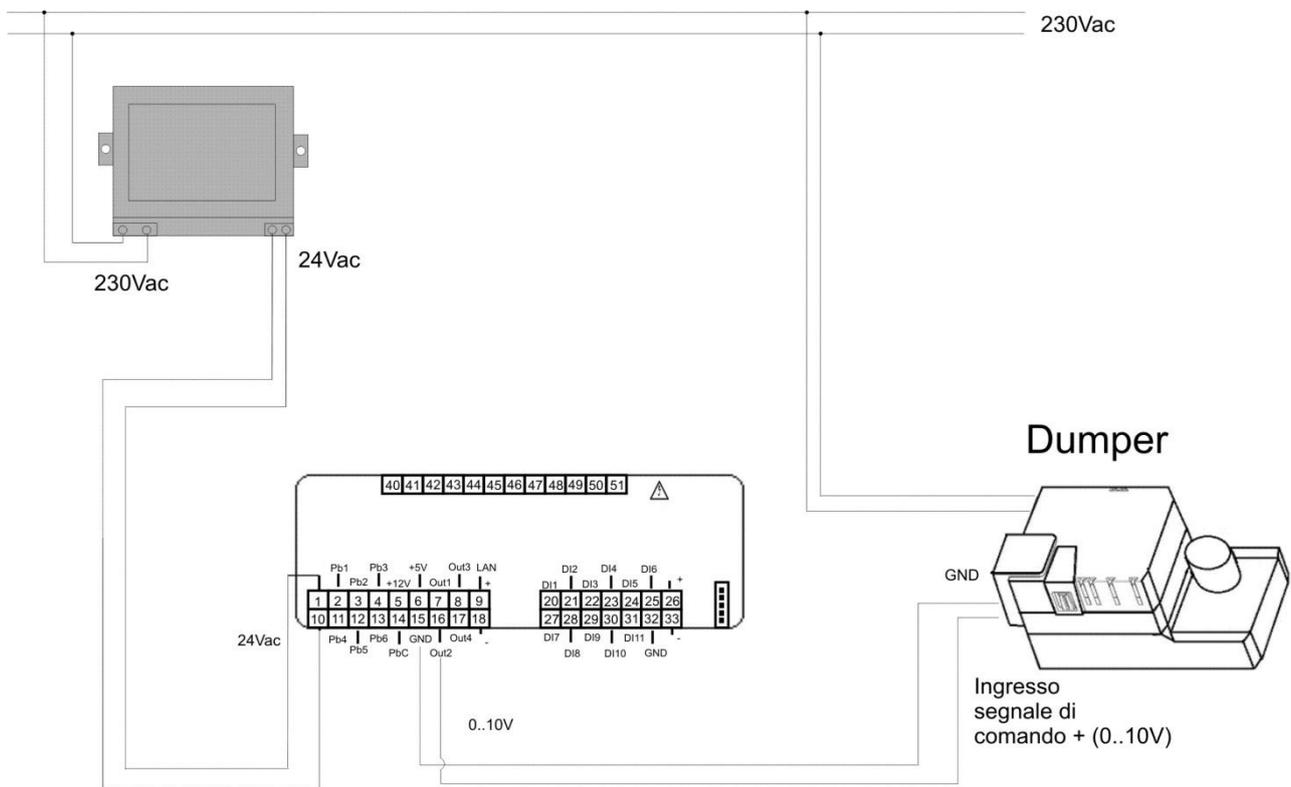
If the dumper motor has a common line between a pole of the power supply and the “-” pole of the 0..10V signal, it is necessary to use two transformers for the power supply of the controller IC200CX and the power supply of the dumper motor.
